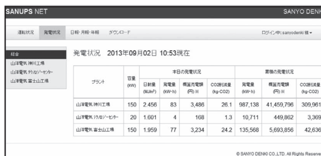
Fig. 2: Screen displaying power generation status of all plants
